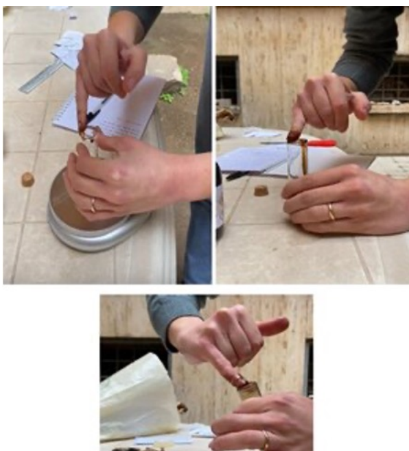
Figure 12: Coating each rim with bitumen (photo taken by the author).
