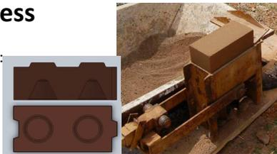
**The Float-Ram** adopts the concept of the floating mould, the process of block forming develops in 4 phases, switching between two different conditions of the machine:
